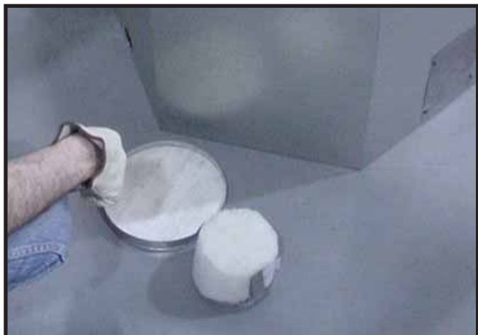
Figure 9.11 Discard the seal cap, remove and discard the insulation basket. Note: Once the vent cap has been removed it CANNOT be reattached.
